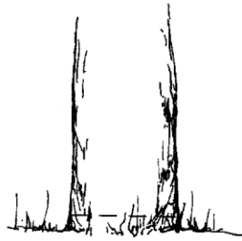
Measure at ground line when reasonable
